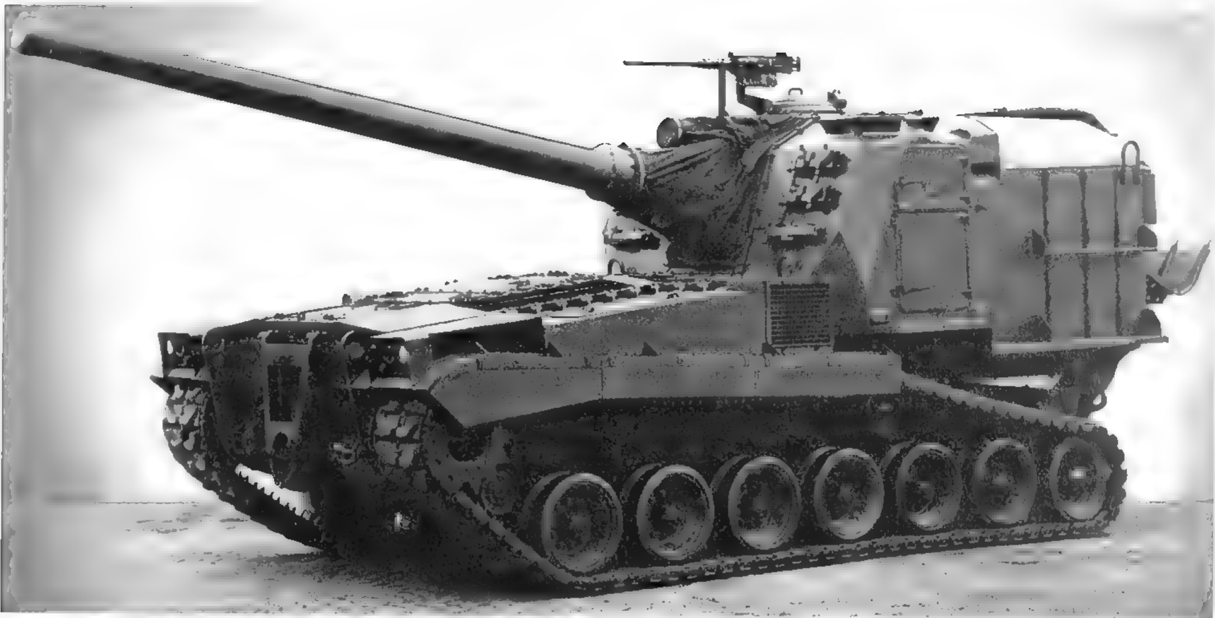
The M53 can be distinguished from the M55 most readily by the length of the gun tube. The M53's 155mm barrel extends beyond the end of the hull as seen here, where the 8-in. armed M55 does not. (Photo courtesy of the Patton Museum)
